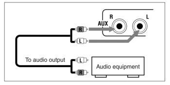
For playing other equipment through this unit, connect between the audio output jacks on the other equipment and AUX jacks by using audio cords (not supplied).
